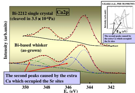
Fig.2 Ca-2p XPS spectrum obtained from the surface of the as-grown whiskers and the Bi-2212 single crystal cleaved in high vacuum ( $3.5 \times 10^{-6} \text{ Pa}$ ) [ $h\nu=4750 \text{ eV}$ ].
