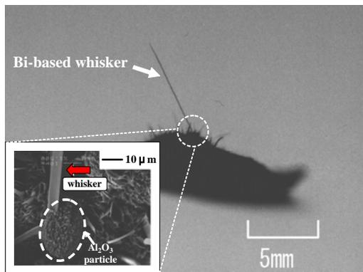
Fig.1 Optical photograph and SEM image of the grown whiskers.
